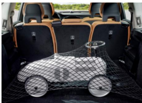
Load Securing Net - Load Compartment
