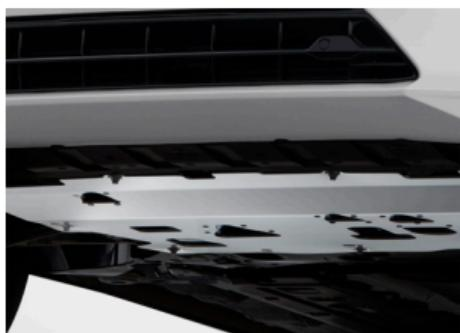
Protective Plate Beneath Engine.
