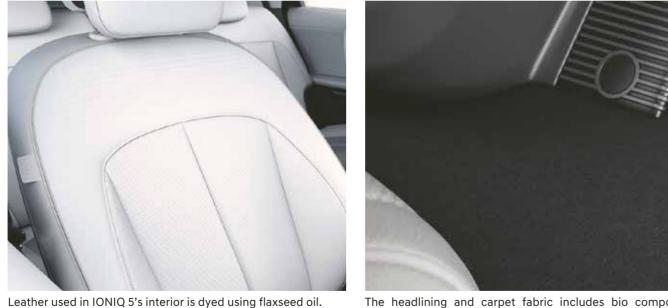
The headlining and carpet fabric includes bio components extracted from sugarcane and corn.
