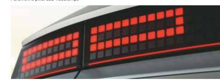
Parametric pixel LED taillamps
