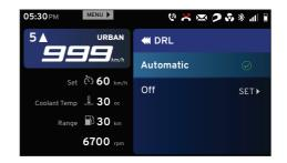
When headlamp switch is in 'Low beam' position the headlamp glows as DRL. But if the 'DRL' is turned 'OFF', the headlamp glows as 'Low beam'.
