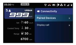
Press the 'Down' (D2) arrow of the control switches (ref. Fig. 24) and press the 'ENT' (D1) button after selecting the to 'Pair a new device' option.
