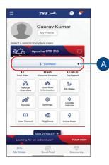
Press and hold the 'CONNECT' tab for 2 secs to erase previous vehicle details if required and connect with a new vehicle in the TVS connect app. • Press 'YES' tab to erase the previous vehicle details or 'NO' to continue as it is.
