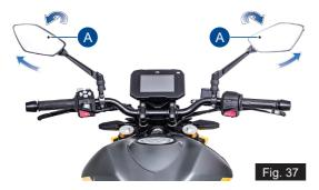
• Tilt the mirror portion (A) till the clear vision is obtained (forward or backward / up or down).
