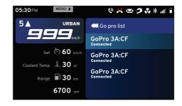
Incase there is no device is paired with the instrument cluster, the message 'currently there is no go pro devices' will be displayed as shown below.
