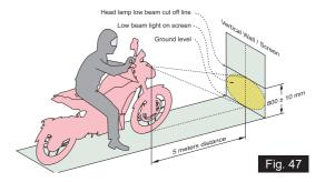
Now, turn the headlamp to low beam mode and ensure the headlamp low beam focus falls between 800 ± 10 mm from the ground level as shown (ref. Fig. 47).
