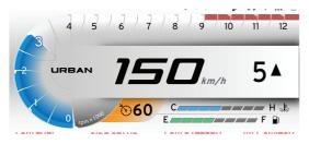
• Digital bands are indicated in blue and red band based on the engine coolant temperature. Refer bellow table for details.
