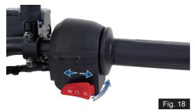
The operation of integrated electric starter cum engine kill switch is explained below:
