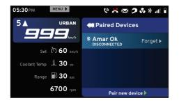
Incase there is no device connected to the TFT instrument cluster, the cluster displays the message 'Currently there is no paired devices' as shown.
