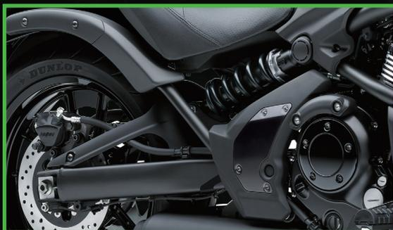
Offset laydown rear single-shock suspension is a distinctive and trend-setting styling element.
